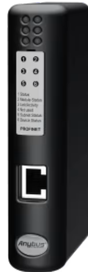
A protocol converter that connects CANopen devices to PROFINET-IO PLCs
