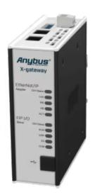
A protocol converter that connects EtherNet/IP and FIPIO control systems
