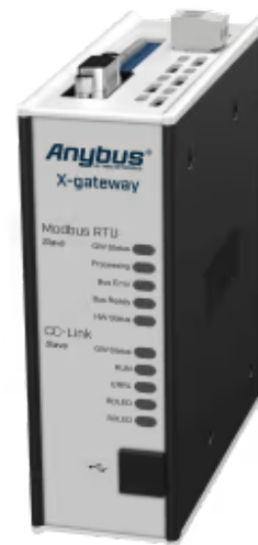
A protocol converter that connects CC-Link and Modbus RTU control systems
