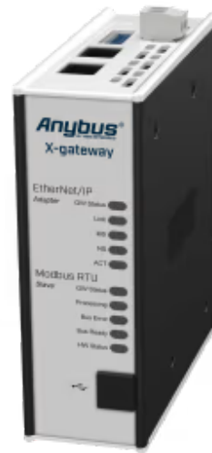
A protocol converter that connects EtherNet/IP and Modbus RTU control systems
