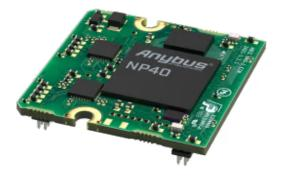
Enable communication between industrial devices and PROFIBUS networks
