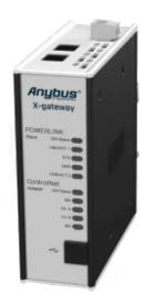
A protocol converter that connects ControlNet and POWERLINK control systems
