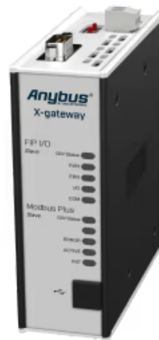
A protocol converter that connects FIPIO and Modbus Plus control systems
