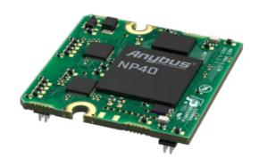
Enable communication between industrial devices and POWERLINK networks
