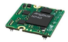
Enable communication between industrial devices and CANopen networks
