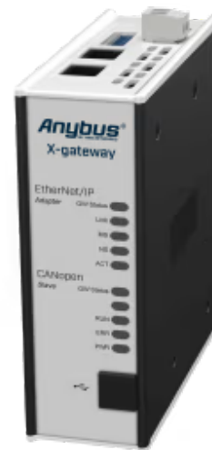
A protocol converter that connects EtherNet/IP and CANopen control systems
