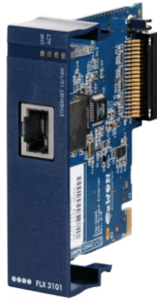
Interchangeable extension card for enhanced connectivity
