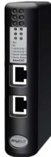
A protocol converter that connects CANopen devices to EtherCAT PLCs
