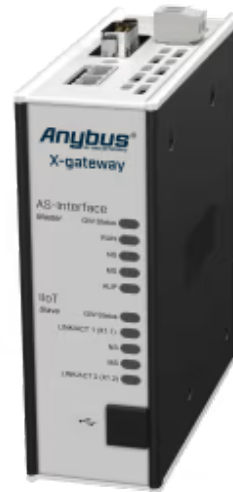
A protocol converter that connects AS-Interface devices to OPC UA-MQTT PLCs
