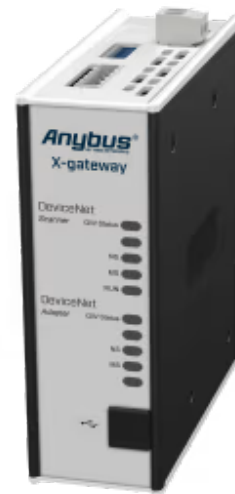
A protocol converter that connects DeviceNet devices to DeviceNet PLCs
