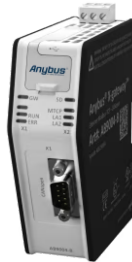
A protocol converter that connects Modbus TCP devices to CANopen PLCs
