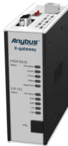
A protocol converter that connects FIPIO and PROFIBUS control systems
