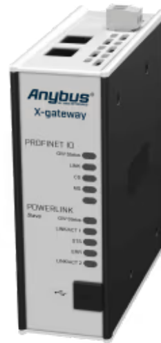
A protocol converter that connects PROFINET-IRT and POWERLINK control systems
