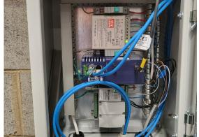
Connecting a laser distance sensor to an Ewon HMS gateway provides precise, real-time measurement and remote control of machine parts. The gateway collects data via Ethernet/IP and securely transmits it using encrypted MQTT protocols.
