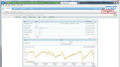
VRTX's systems for cooling water are controlled by a PLC. A Netbiter gateway is connected to the PLC and sends data via the mobile network to Netbiter Argos. By logging into www.netbiter.net, VRTX and their customers can monitor and control their systems.
