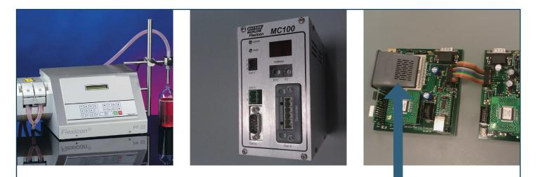
MC100 handles a closed loop system. Filling weight signals for automatic recalibration of individual fillers can be sent via an existing PLC.
