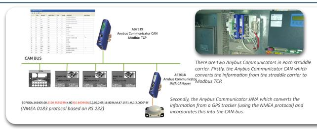
deemed that the Anybus Communicator CAN would be a perfect fit to handle the conversion between the CAN-based network in the 22 straddle carriers and the Modbus-TCP network. The Anybus Communicator CAN works as a translator between the CAN-bus in the straddle carrier and the Modbus TCP of the communication system, converting each telegram through built-in hardware and software. Together with PICS, APM Terminals started mapping the communication between the CAN-bus and the monitoring system.
