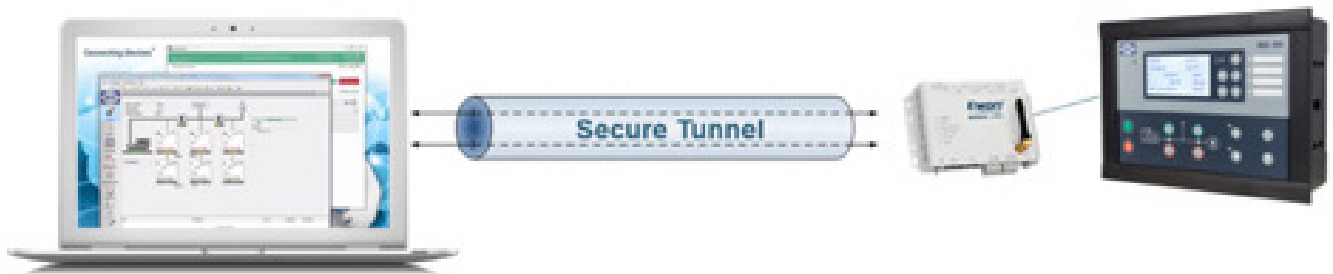
A remote access connection of DEIF controllers enabling using DEIF utility software remotely.
