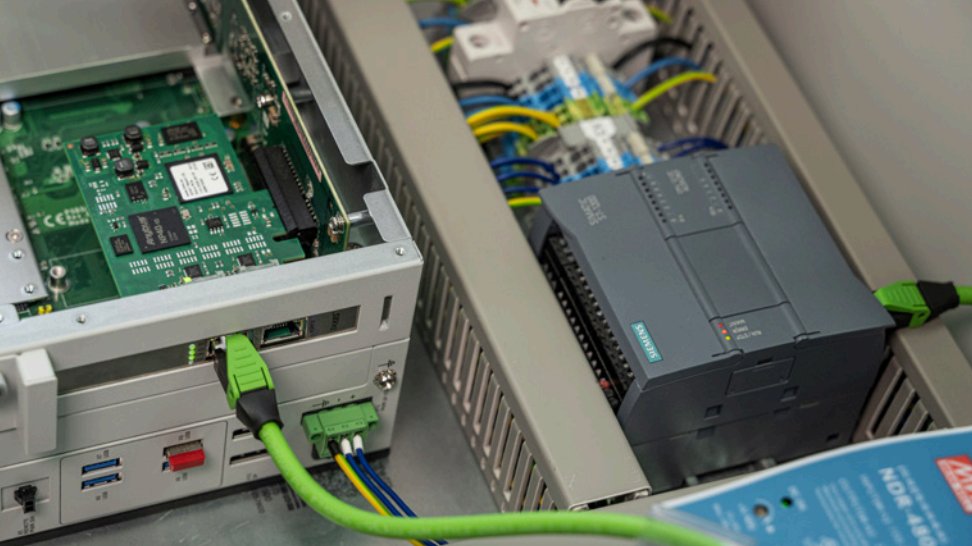
Left: Connecting the Sarissa Box-PC to the PLC with Ixxat INpact.
