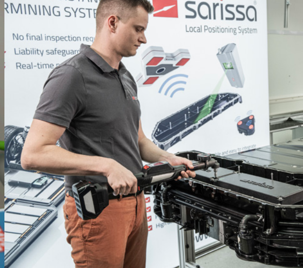
Right: Determining the position of the hands and handheld tools in 3D with hand transmitter or tool module.
